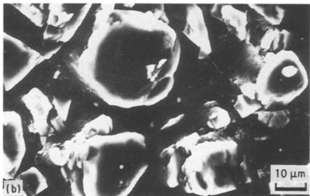
Figure 3 Scanning electron micrographs of metallographically polished surfaces of (a) LM11-SiC fibre, and (b) LM11-SiC particle composites.
