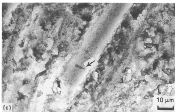
Figure 4 Abraded surfaces of the LM11-SiC fibre composite showing (a) pull-out of SiC fibres at 49 N, and (b, c) the protrusion of SiC fibres at 22 N. The weak fibre/matrix interface (b) and microcrack in a fibre generated during abrasion (c, arrowed) may be noted.
