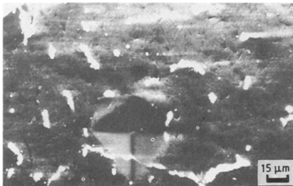
Figure 8 A typical microhardness indentation mark in the subsurface region. Note: the upper half of the mark closer to the abraded surface (top) is less than the lower half.
